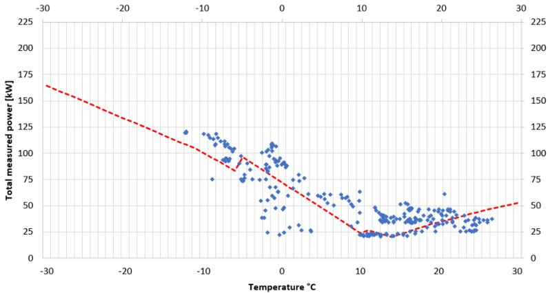
Figure 8.3: X61 Active parking - Recorded total auxiliary power at different ambient temperatures (blue dots) and simulated power curve for the same span (red dashed line)
