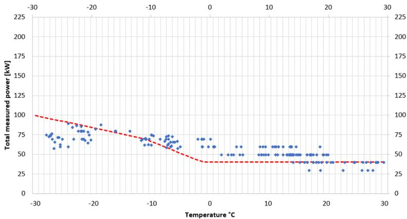
Figure 8.2: X55 Parking mode - Recorded total auxiliary power at different ambient temperatures (blue dots) and simulated power curve (red dashed line)
