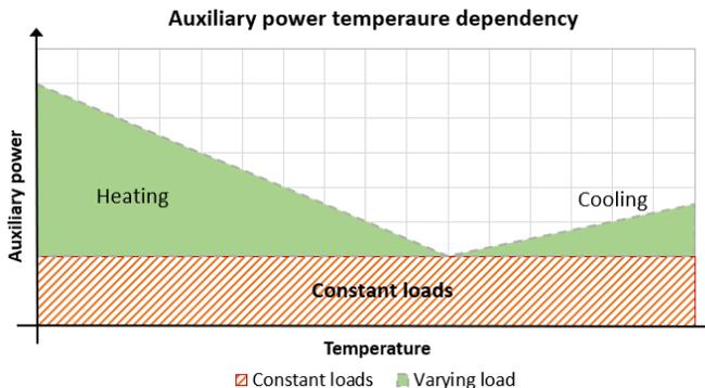
Figure 4.2: Example of total auxiliary power need with an ambient temperature dependent varying load.
