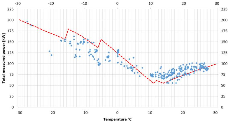
Figure 8.1: X55 Active mode - Recorded total auxiliary power at different ambient temperatures (blue dots) and model power curve (red dashed line)
