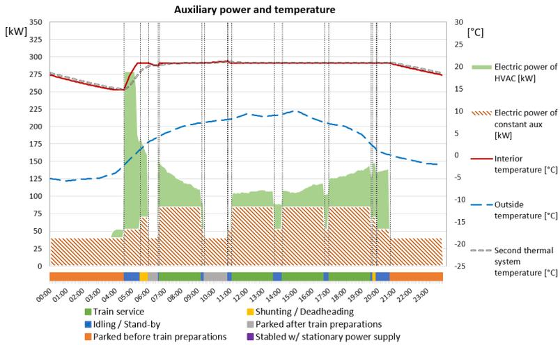
Figure 7.7: Auxiliary power use for a X55, temperature and operational situations. Simulated for type day 2, cold spring weather, with operation between Malmö and Göteborg.
