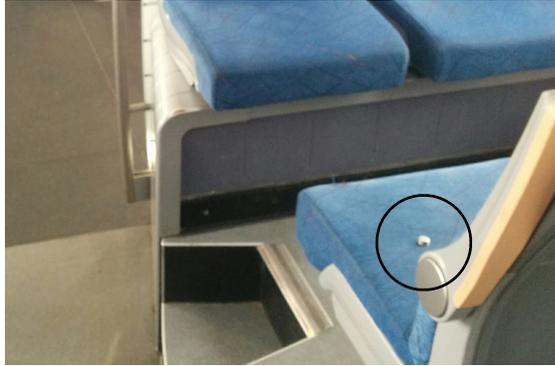
Figure 7.1: I-button temp-logger placed inside a X61 in Sävenäs
