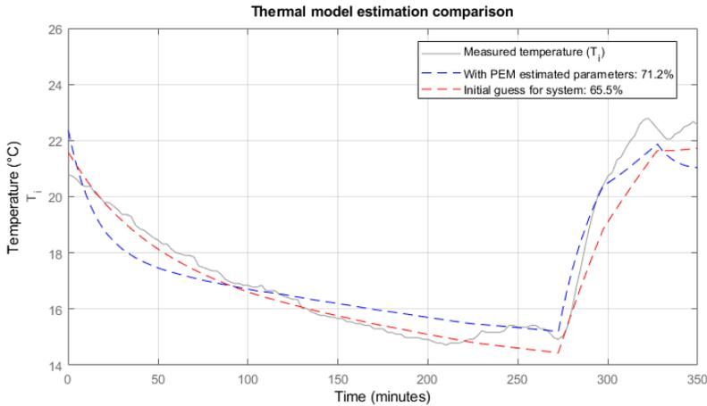
Figure 7.2: Example of PEM-estimation fit on data for one of the cool down heat up tests, performed on an X61 in Sävenäs
