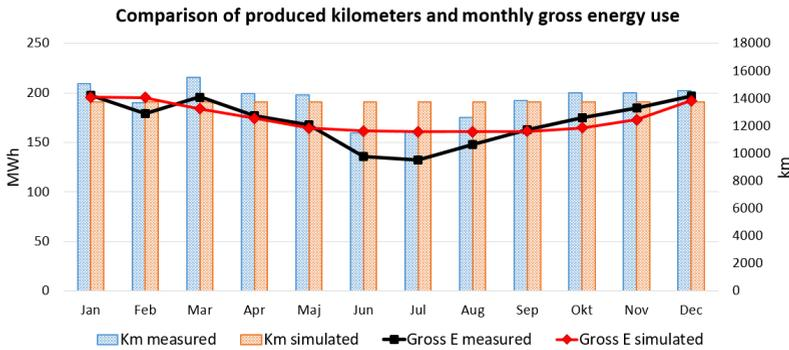
Figure 8.7: X61 - Produced kilometers (bars) and monthly energy use (lines) for simulation and reference year.
