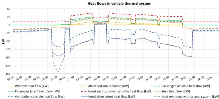
Figure 7.10: Stacked line plot of heat flows in vehicle thermal system. For X55 simulated for type day 2, cold spring weather.
