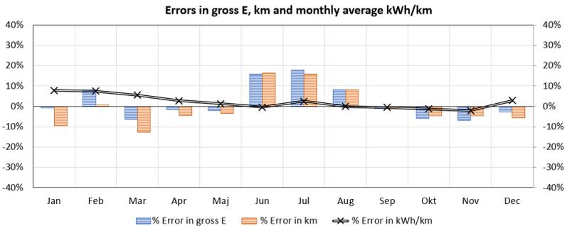
Figure 8.9: Monthly errors in simulated energy, kilometres and kWh/km for one X61 train, compared with reference data
