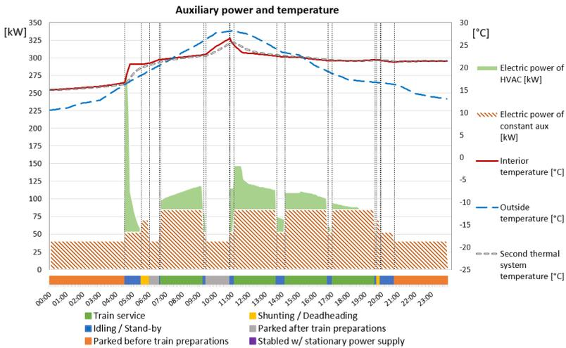
Figure 7.8: Auxiliary power use for a X55, temperature and operational situations. Simulated for type day 2, warm summer weather, with operation between Malmö and Göteborg.
