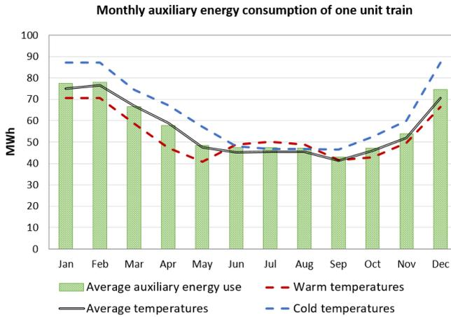
Figure 7.13: Monthly variations in auxiliary energy use for a X55 train. Simulated for a year with the *average operational cycle*
