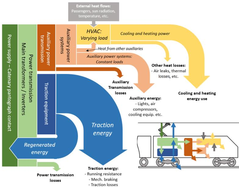
Figure 4.1: Energy flow diagram of a passenger rail vehicle, including heat flows affecting the HVAC energy use.
