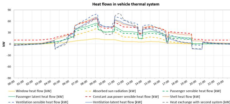
Figure 7.11: Stacked line plot of heat flows in vehicle thermal system. For X55 simulated for type day 2, warm summer weather.
