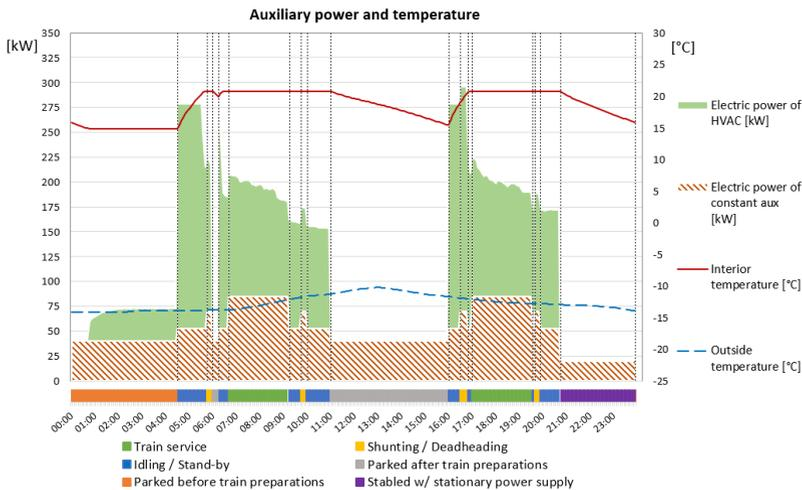
Figure 5.1: Simulated auxiliary power need for a X55 train going through a winter day. The coloured bar at the bottom illustrates the different operational situations the train is going through. The auxiliary power is made up of the two parts, the constant (striped red) and the varying (green) components. The ambient temperature as well as the vehicles interior temperature are also plotted in same figure<sup>7</sup>
