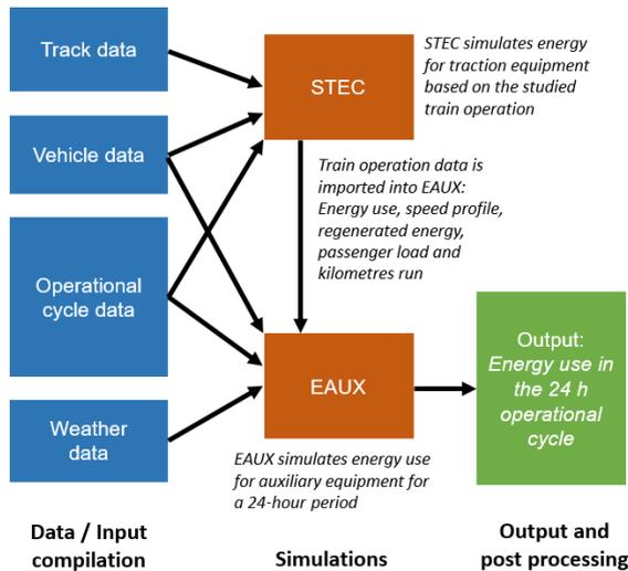
Figure 6.2: Simulation work flow
