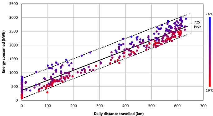
Figure 2.1: Energy use plotted against the daily travel distance and ambient temperature in the case of the T&W Metro [11].
