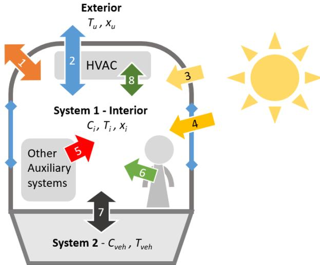
Figure 6.1: Illustrated representation of the vehicle thermal model
