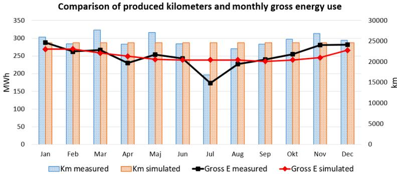
Figure 8.6: X55 - Produced kilometers (bars) and monthly energy use (lines) for simulation and reference year.
