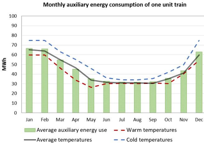
Figure 7.14: Monthly variations in auxiliary energy use for a X61 train. Simulated for a year with the *average operational cycle*
