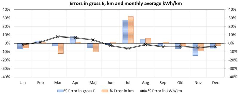
Figure 8.8: Monthly errors in simulated energy, kilometres and kWh/km for one X55 train, compared with reference data
