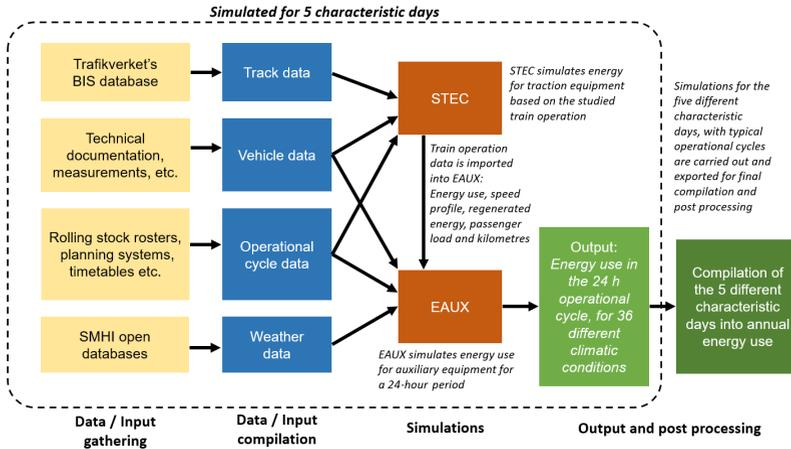
Figure 7.6: Work flow for case study simulations (based on the general simulation workflow previously shown in Figure 6.2)
