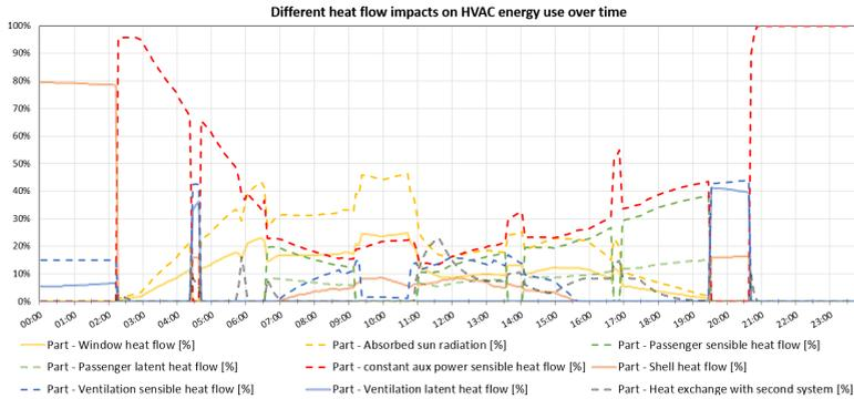
Figure 7.12: The different heat flows influence in percent on the varying auxiliary load over time on a X55. Simulated for type day 2, warm summer weather.
