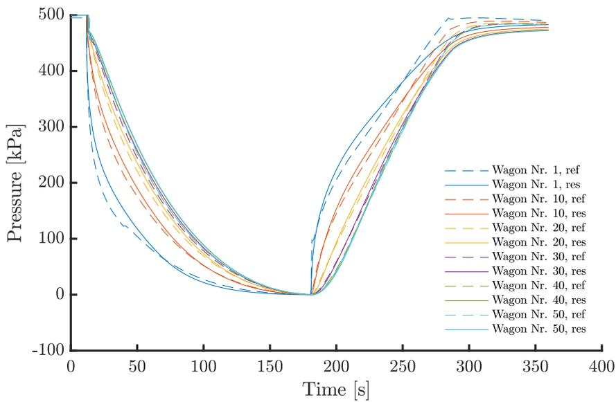
Figure 5.7 – MP pressure profiles of emergency application measurement and corresponding simulation after first calibration step, test train length 750 m.
