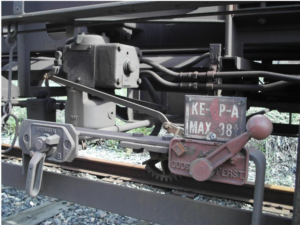
Figure 2.2 – DV, switch handles and piping mounted on a freight wagon.
