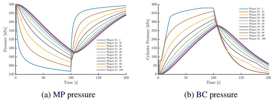
Figure 4.9 – Example of brake release during ongoing application on a 1.5 km train.
