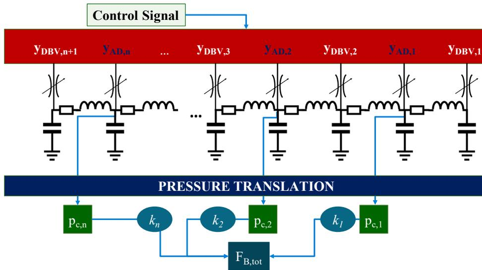
Figure 4.5 – Model structure of the equivalent electric circuit hybrid,  $n$  wagons.
