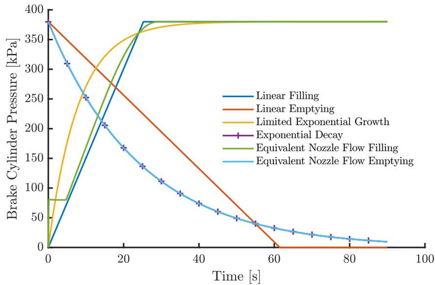
Figure 4.4 – Three variants of limiting curves for delayed brake application and release, in brake type G.
