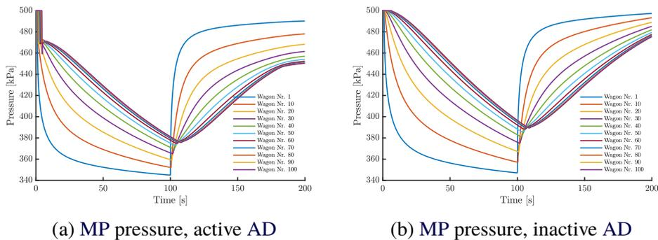
Figure 4.11 – Comparison of brake application with and without **AD** on a 1.5 km train.
