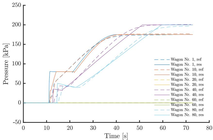
Figure 5.10 – BC pressure profiles for measurement of pressure propagation and simulation after calibration, train length 1200 m, brake type G.
