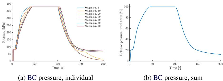
Figure 5.5 – BC pressure profiles for full service brake application and release on the iron ore train, individual and sum of all pressures in relative terms.
