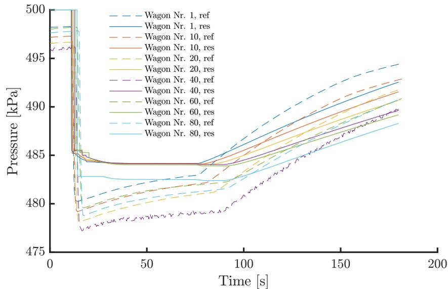
Figure 5.12 – R pressure profiles for measurement of minimal brake application, simulation after calibration, train length 1200 m, brake type G.
