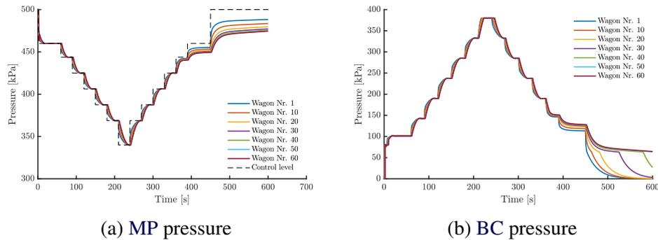
Figure 4.10 – Example of gradual brake application and release on a 746 m train with brake type G.
