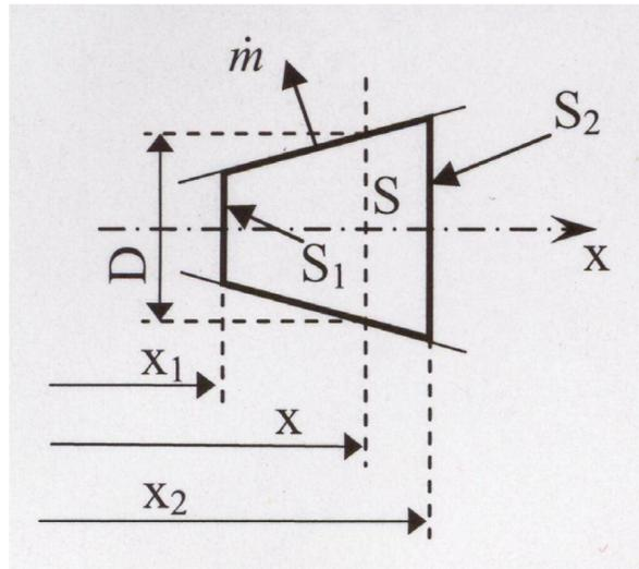
Figure 2.5 – Schematic view of the pipe model used in TrainDy. Source: [24]
