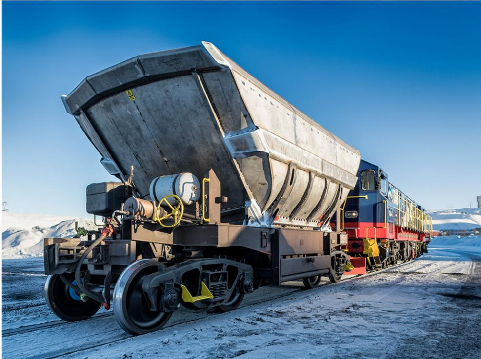
Figure 1.2 – Ore wagon with visible BC, lever mechanism, R and coupling hose. *Photo: Fredric Alm / Kiruna Wagon*
