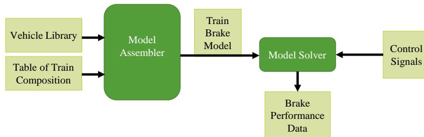
Figure 3.1 – Functional framework structure of the test bench.
