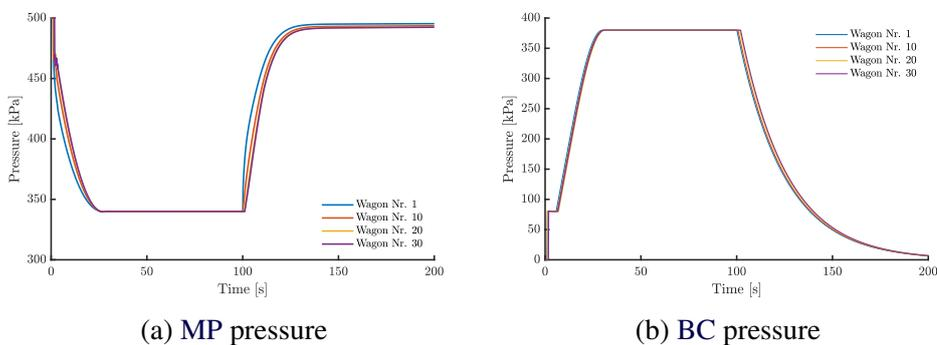
Figure 5.1 – Pressure profiles for full service brake application and release on the steel commuter train.
