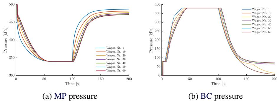
Figure 5.2 – Pressure profiles for full service brake application and release on the iron ore train.
