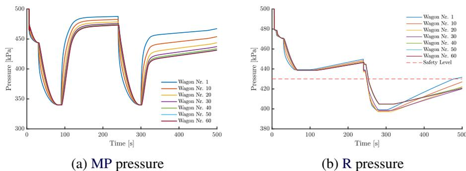
Figure 5.3 – Pressure profiles for two consecutive service brake applications and releases on the iron ore train.
