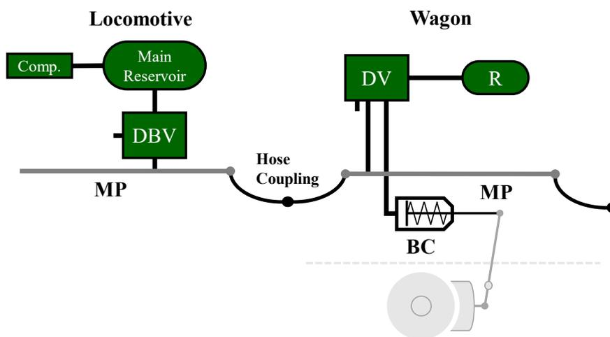
Figure 2.1 – System layout of the UIC air brake system for freight trains.
