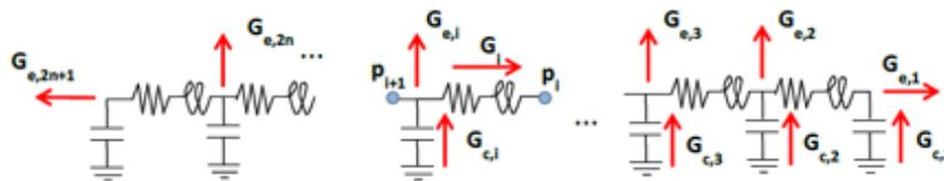
Figure 2.4 – Equivalent electric circuit setup of the pneumatic model used in the *DYNAFREIGHT* project. Source: [27]
