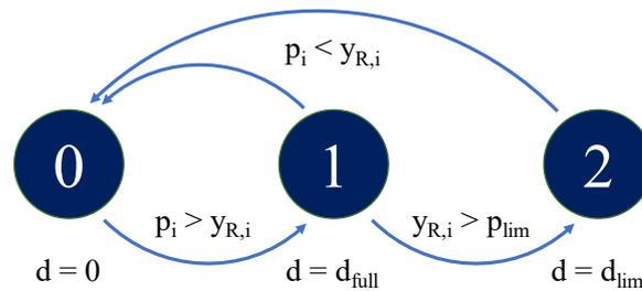
Figure 4.7 – Graphical representation of the state machine logic for the filling of R.
