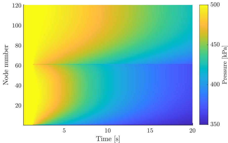
Figure 4.3 – Pressure reduction in the MP of a 900 m long train consisting of 60 wagons. A second locomotive is located in the middle of the train.
