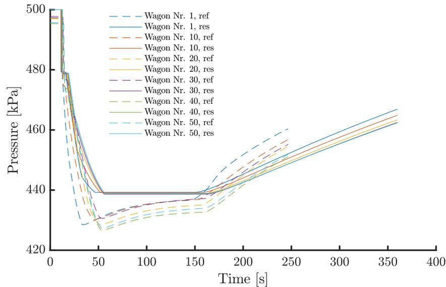
Figure 5.11 – R pressure profiles of full service application measurement and simulation after calibration, test train length 750 m, brake type P.
