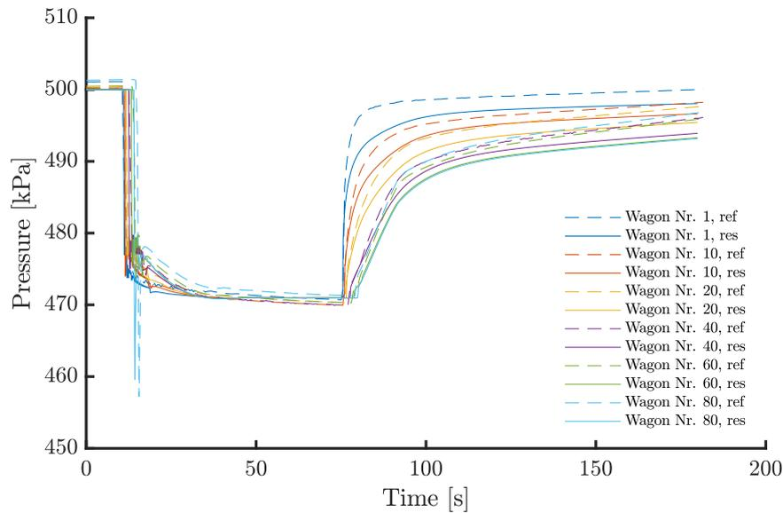
Figure 5.8 – MP pressure profiles for measurement of minimal brake application and simulation after calibration, train length 1200 m.
