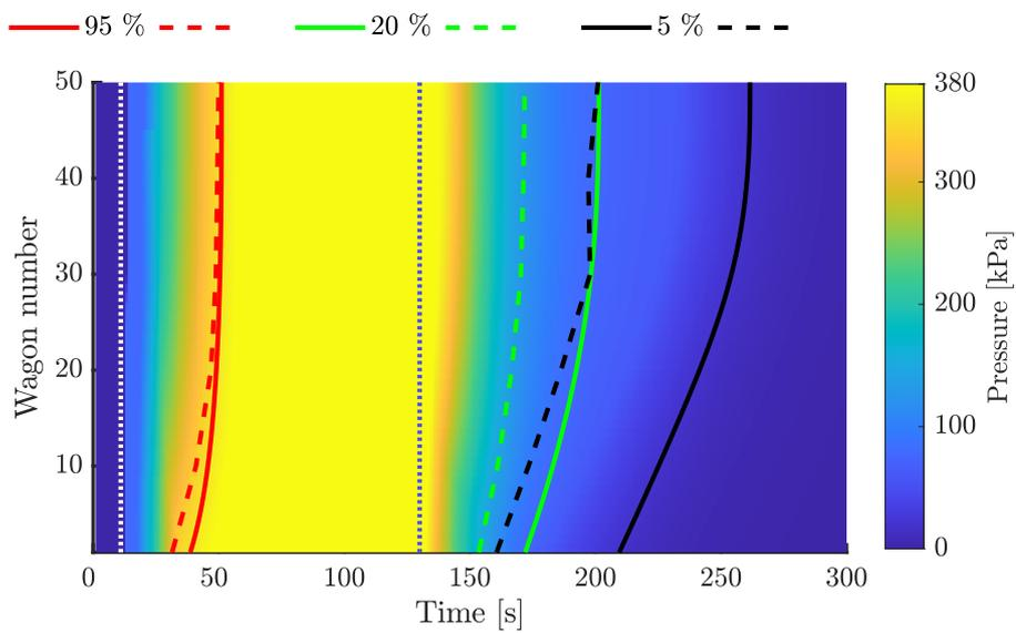
Figure 5.14 – Timing curves for BC pressure, full application and release, train length 750 m, brake type P. Dashed lines indicate reference values.
