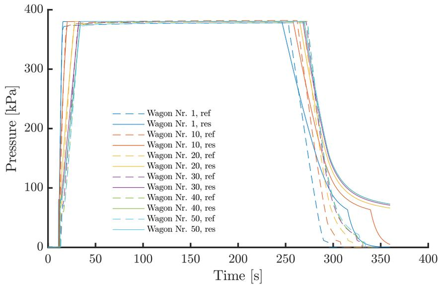
Figure 5.9 – BC pressure profiles of emergency application measurement and simulation after calibration, test train length 750 m, brake type P.
