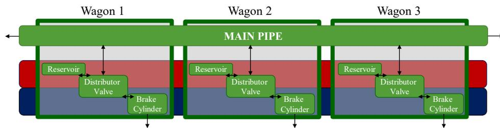
Figure 4.2 – Modular structure from a solution perspective.
