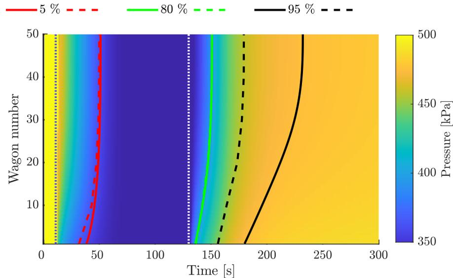
Figure 5.13 – Timing curves for MP pressure, full application and release, train length 750 m, brake type P. Dashed lines indicate reference values.
