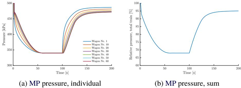
Figure 5.4 – MP pressure profiles for full service brake application and release on the iron ore train, individual and sum of all pressures in relative terms.
