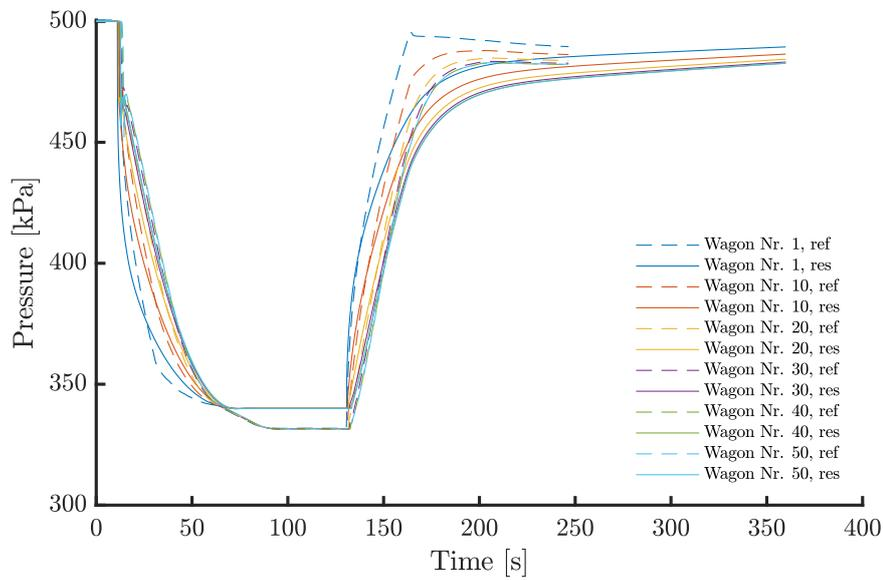
Figure 5.6 – MP pressure profiles of full service application measurement and corresponding simulation after first calibration step, test train length 750 m.
